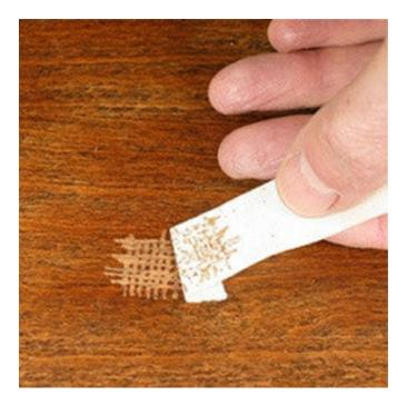
First, score the coating with the razor blade in a crosshatch pattern with about onesixteenth inch between cuts. Then press the masking tape over the cuts rub with an eraser to ensure bonding and pull it up quickly.
