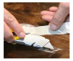
This test is often used at job sites and involves cutting an X into the coating with a sharp knife or other cutting device. A straightedge is used to ensure the cuts are straight. Then, pressure-sensitive tape is placed in the centre of the X and quickly removed. The area is then inspected to see if any coating has been removed from the substrate. These pictures illustrate a failure.
