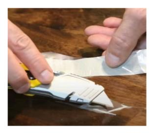
This test is often used at job sites and involves cutting an X into the coating with a sharp knife or other cutting device. A straightedge is used to ensure the cuts are straight. Then, pressure-sensitive tape is placed in the centre of the X and quickly removed. The area is then inspected to see if any coating has been removed from the substrate. These pictures illustrate a failure.
