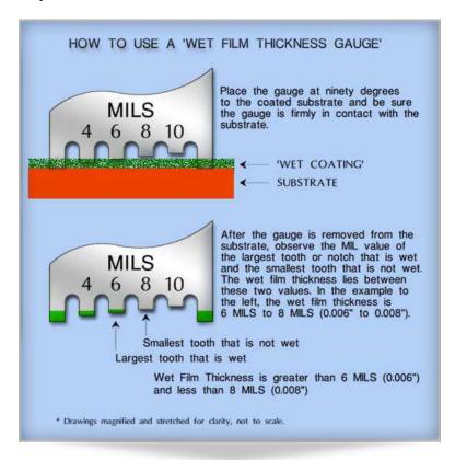
A wet film thickness gauge, or "comb," after touching freshly applied green paint. The arrow points to the estimated wet film thickness, which is the point between the largest coated value and the smallest uncoated value.
