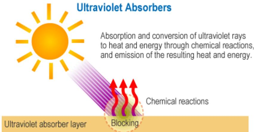
**UVA absorbers** absorb ultraviolet rays (energy) efficiently and dissipate them into heat. This helps to prevent visual and mechanical degradation as a result of photo-oxidation, thereby extending the lifetime of the coating and ensuring a high performance over a long period of time.
